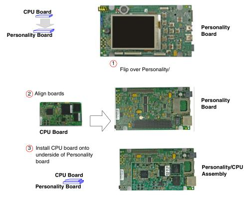
Figure 3.5 Install CPU Board onto Personality Board
